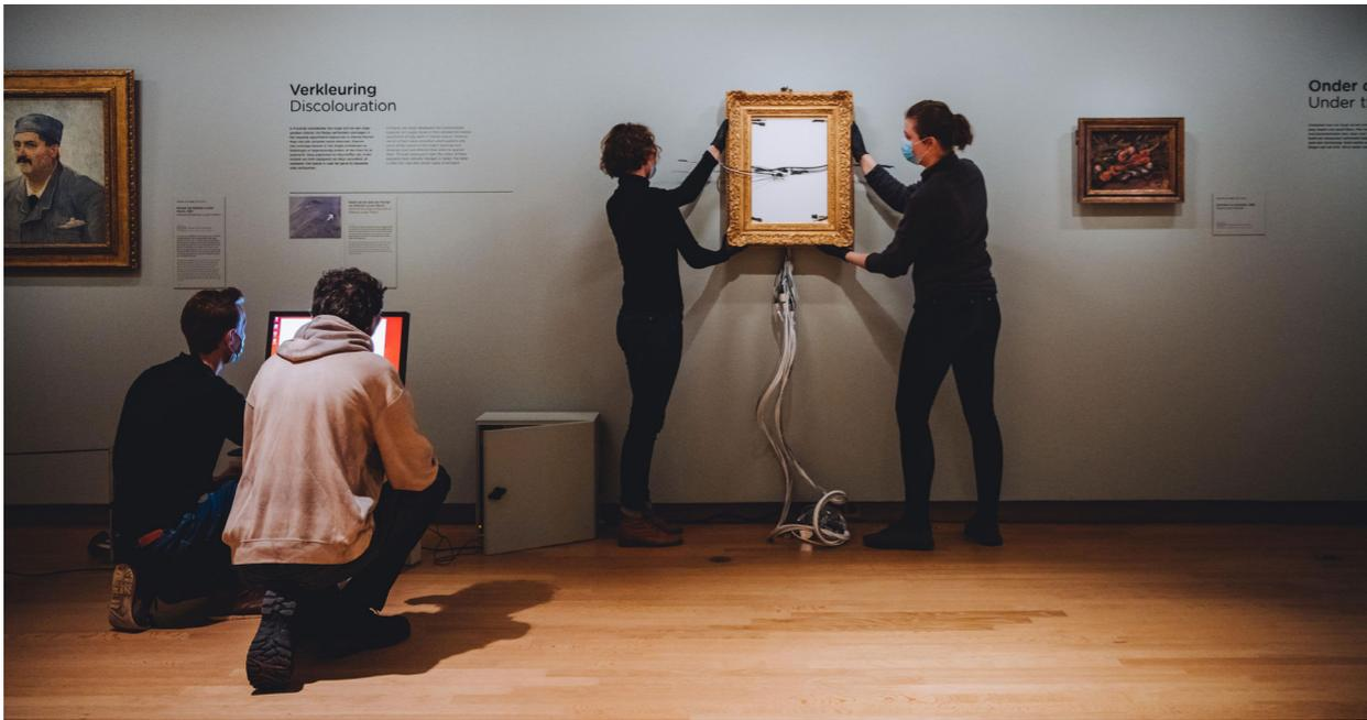
The museum is collaborating with ASML to develop a method to monitor paintings individually. This is a test set-up fitted with 45 sensors that measure temperature, relative moisture and light.
